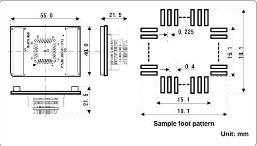
Figure 5.3 External dimensions of the FLX-144NSE
